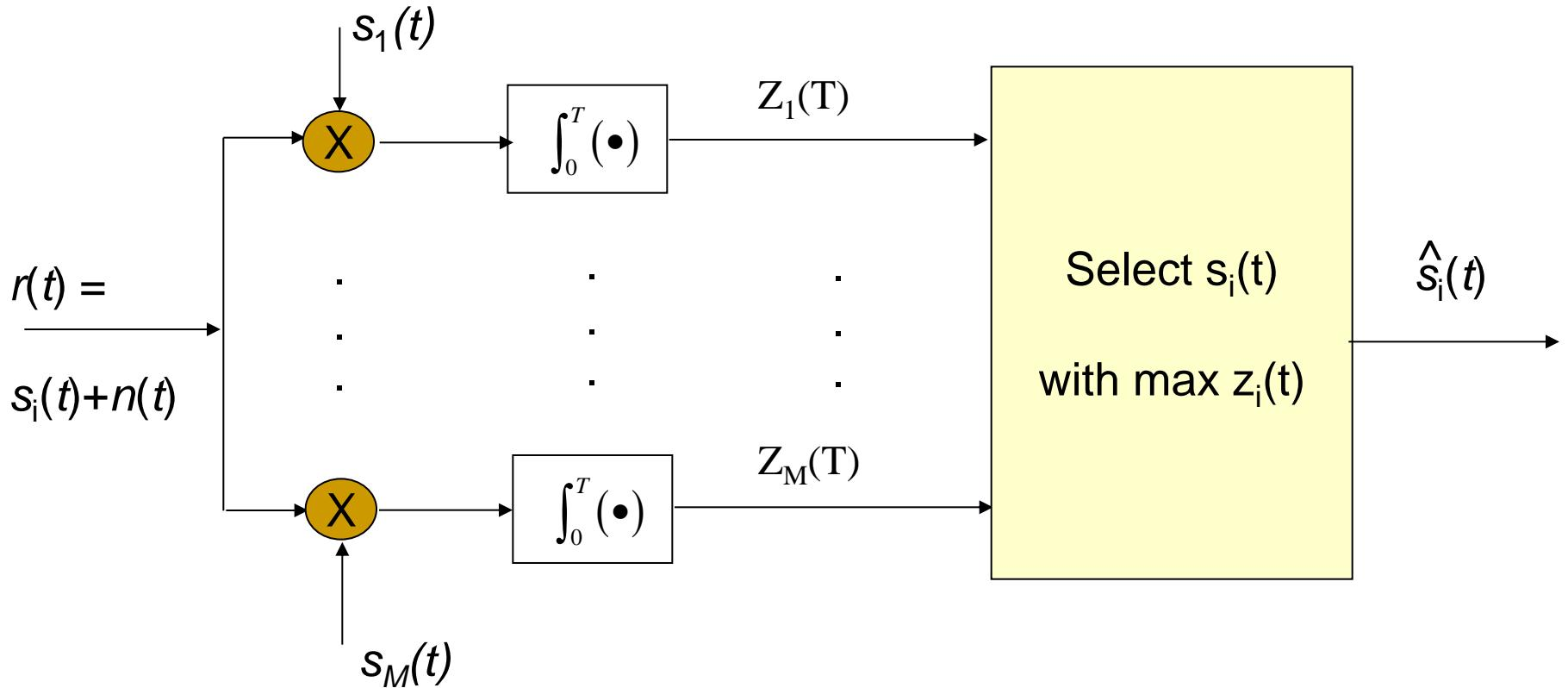
Applies for PSK, FSK, ASK, QAM, etc.
