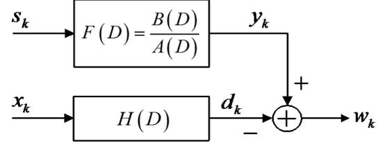
Figure 2. A block diagram for designing the IIR equalizer.
