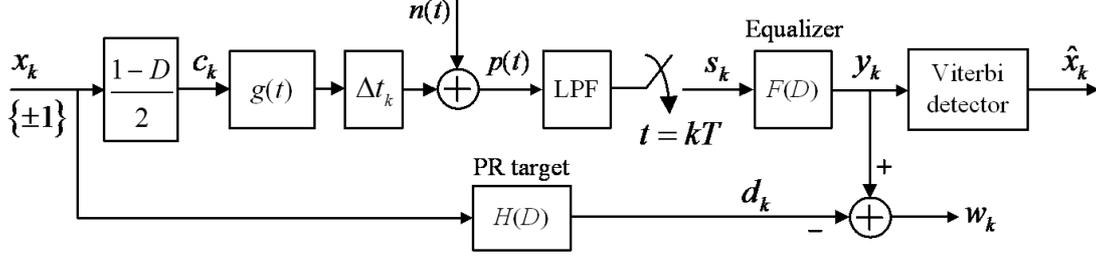
Figure 1. A system model with equalizer design.
