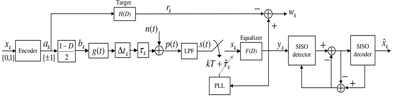
Figure 1: Channel model with target design.
